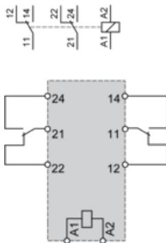
NOTE: For DC input, A1 have to be +, otherwise it would short circuit from protection module
